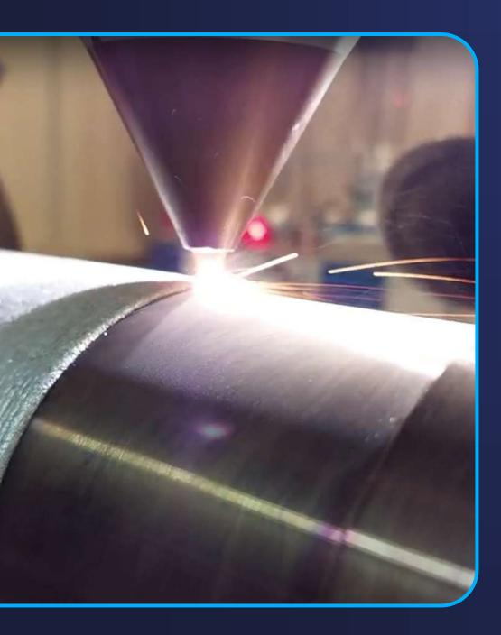
Laser Technology allows us to offer Hardfacing and Hardbanding services with low thermal impact and premium quality, maximizing the useful life of each tool.
